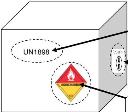
The diagram shows a 3D perspective of a rectangular box. On the front face, there is a label with the text 'UN1898' and a diamond-shaped hazard label with a flame and the text 'ORGANIC PEROXIDE'. On the side face, there is a circular 'UN' marking. Arrows point from these elements to callout boxes.
